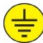
TERMINAL BOARD GROUNDING
