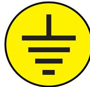
The oven must be included in an equipotential system and connected with a conductor having a minimum wire gauge of 10 mm<sup>2</sup>, connected to the terminal located on the back of the oven bearing the appropriate symbol.
